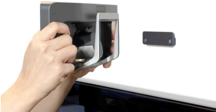
Figure 3. Cisco TelePresence SX10 Wall-Mount Solution
